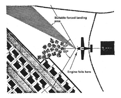
Engine Failure During Takeoff-You are belting along the runway, building up speed and minding your own business when a cessation of activity up front announces there has been an engine failure:
